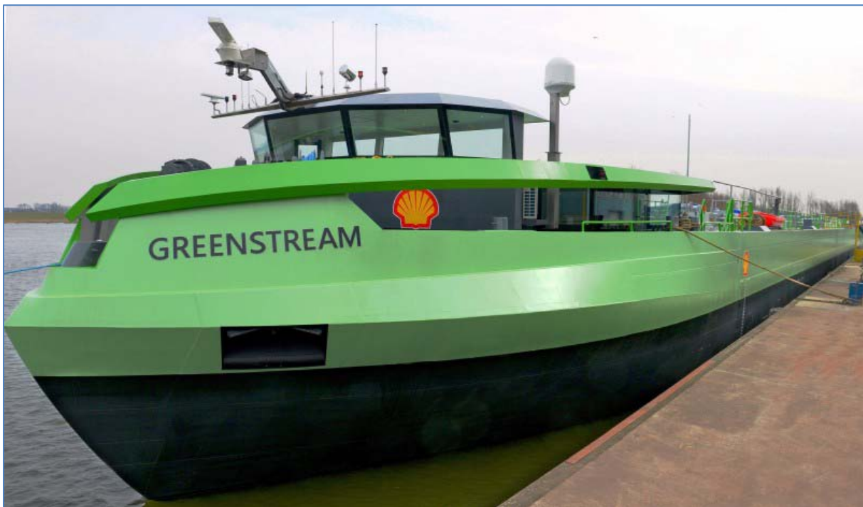
Figure 4 LNG/electric powered tanker. Source: Shell.
