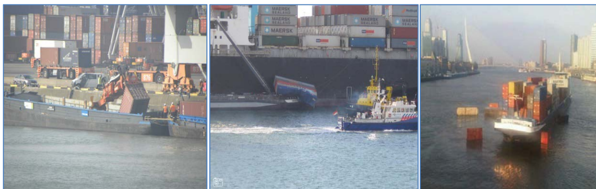
Figure 53 Images of incidents where containers have fallen overboard onto a vessel below.
