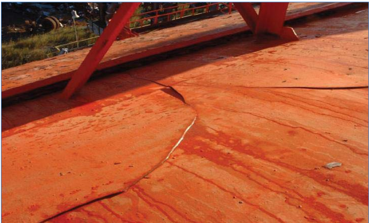
Figure 35 Deck plate cold crack. Source: DNV GL.
