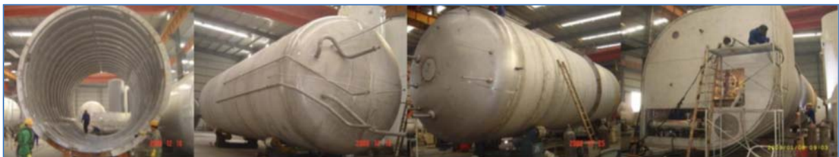
Figure 12 C-class LNG tank vacuum isolated with integrated cold box. Source: Wärtsilä
